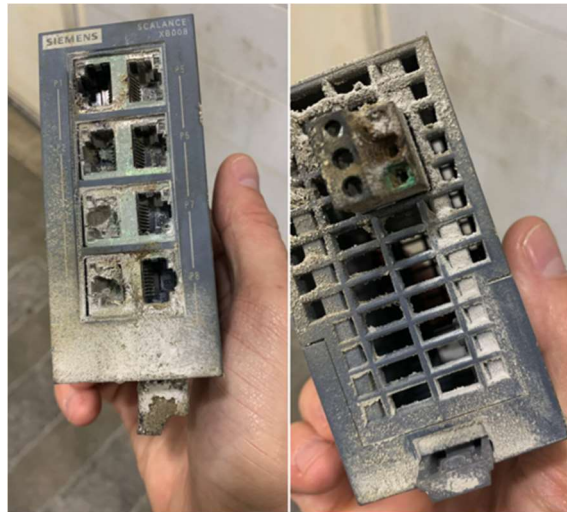
Figure: OT switch being used in environment with lot of dust
